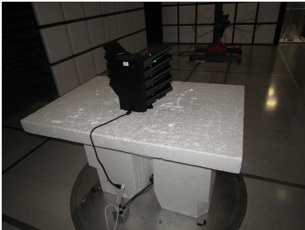
Figure 2: Radiated Emissions – Back View – Below 1GHz
