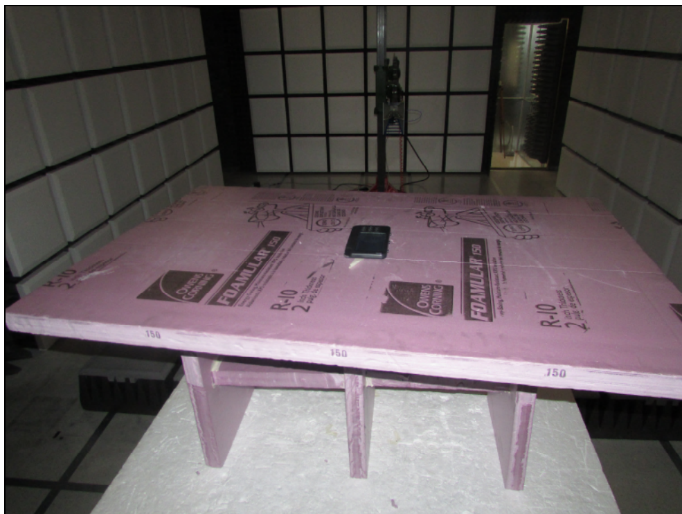
Figure 6: Radiated Emissions – Rear View – Above 1GHz (Wifi)
