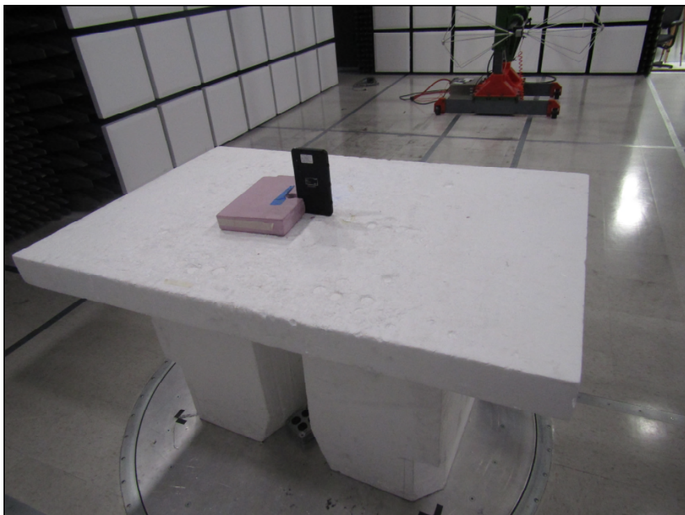
Figure 2: Radiated Emissions – Rear View – Above 30MHz (RFID)
