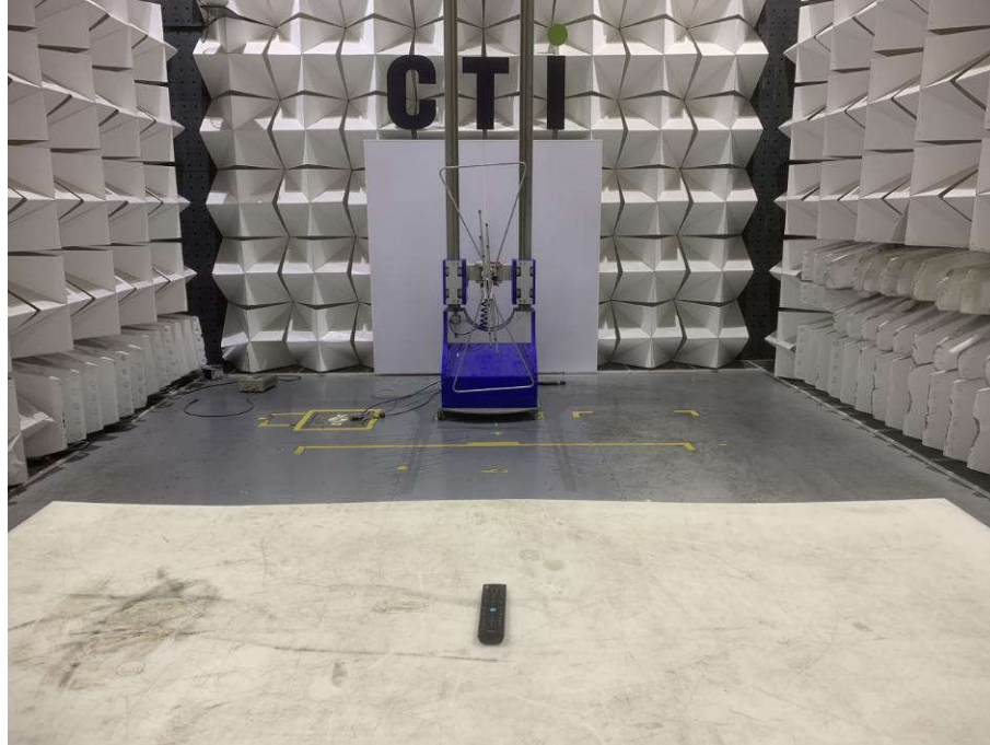
Radiated emission Test Setup-1 (30MHz~1GHz)
