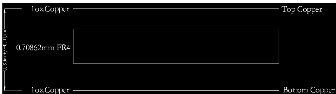
FIGURE 10 PCB LAYER STACK UP
