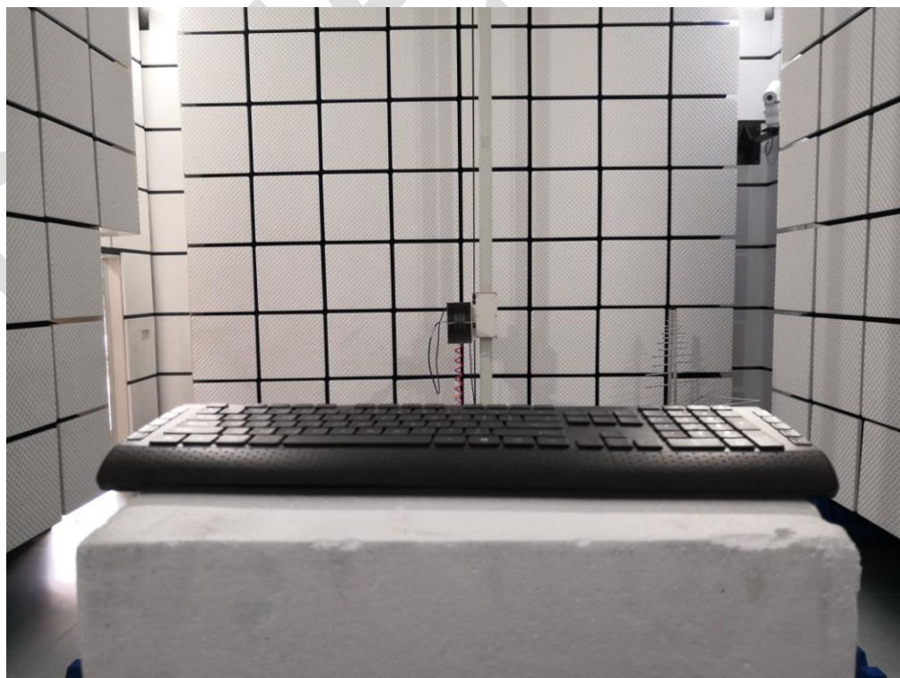
Radiated spurious emission Test Setup-3(Above 1GHz)
