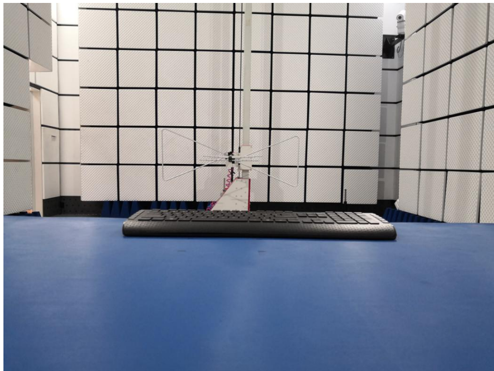
Radiated emission Test Setup-2 (30MHz~1GHz)
