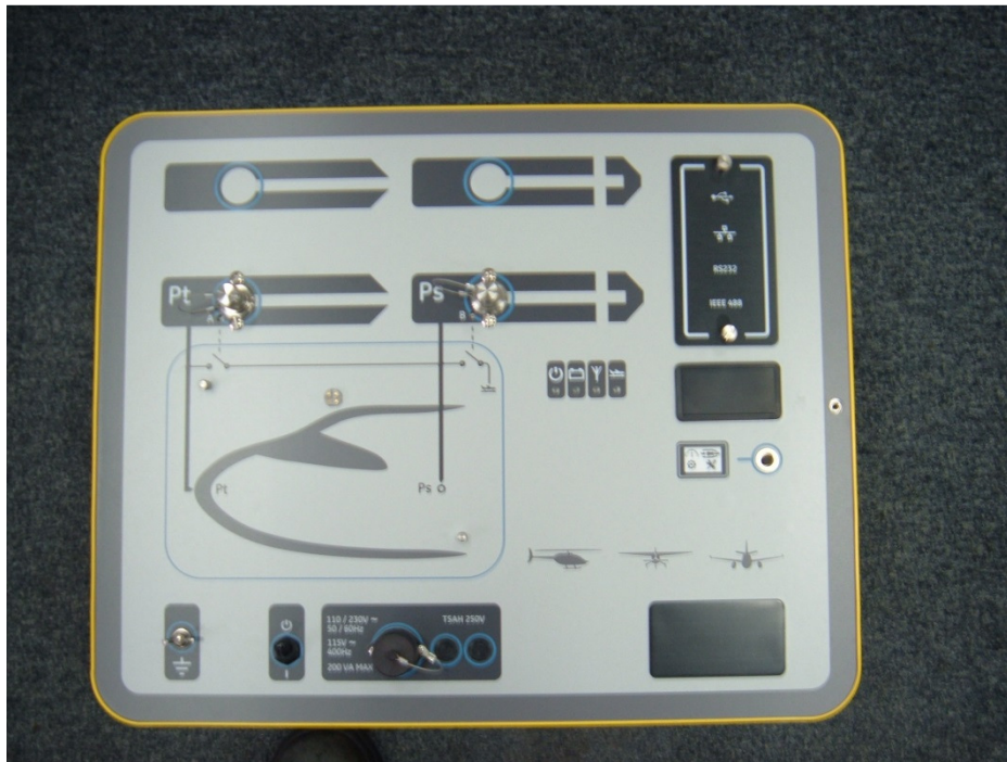
Front Panel with Mains Cable Connected – Patch Antenna Cover Located Middle Right
