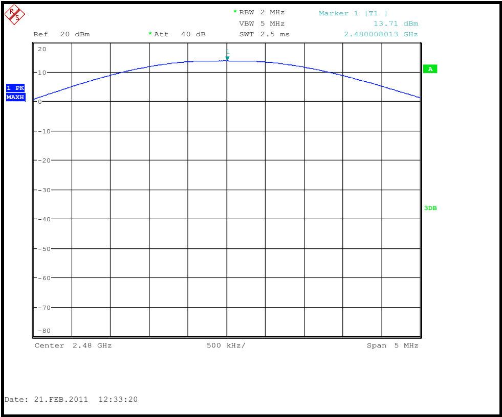
Conducted carrier power 2480.0 MHz – 1Mbps
