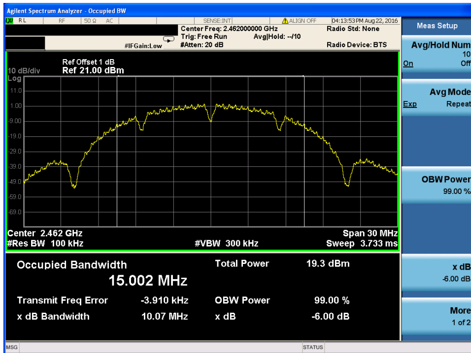
6dB Bandwidth plot on channel 1
