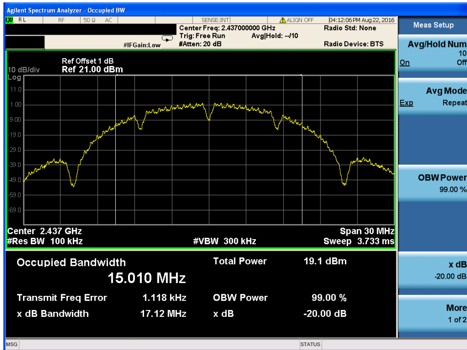
20dB Bandwidth plot on channel 6
