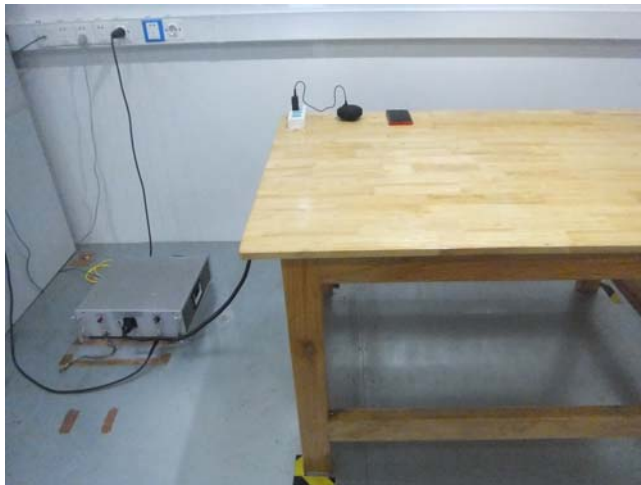
Conducted Emissions Test Setup – Front View
