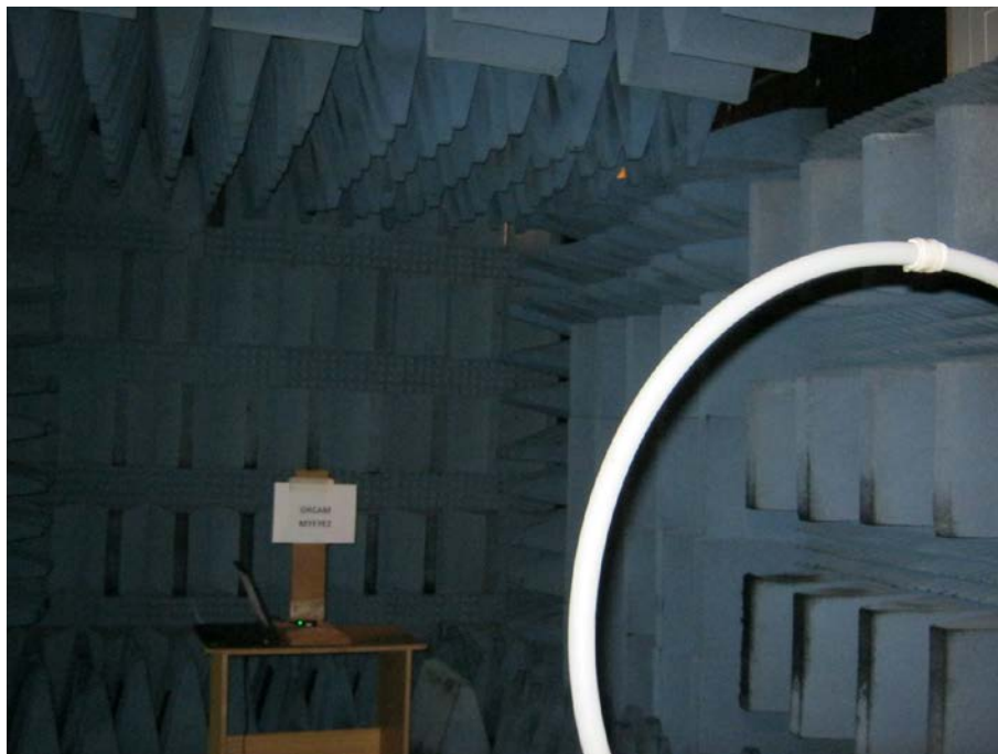
Figure 5. Radiated Emission Test - 0.009-30MHz
