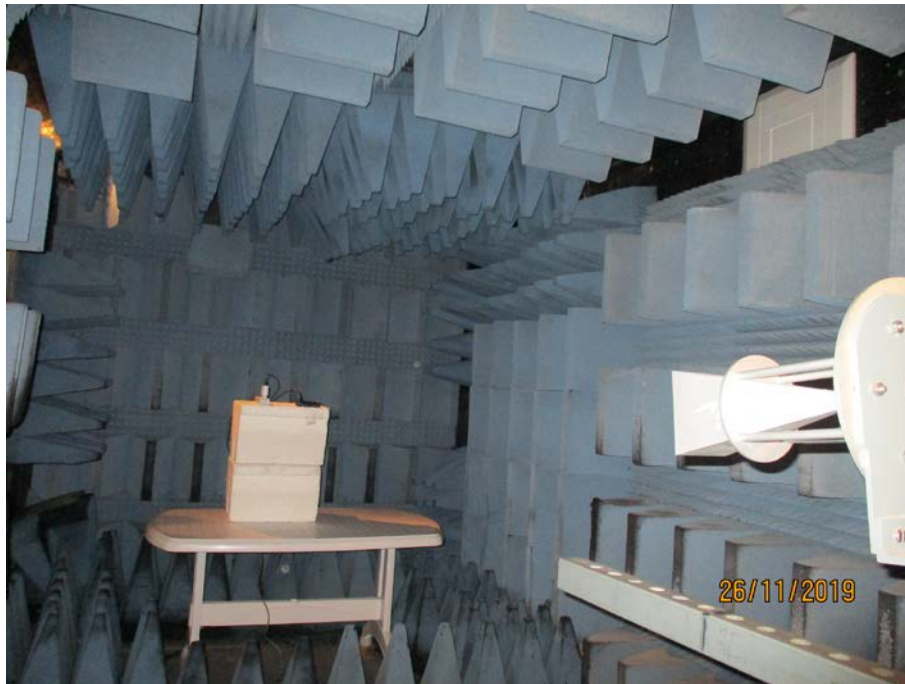
Figure 10. Radiated Emission Test, 18-25GHz
