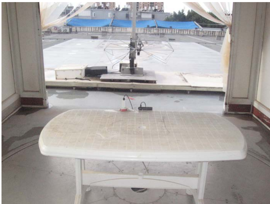
Figure 7. Radiated Emission Test, 30-200MHz
