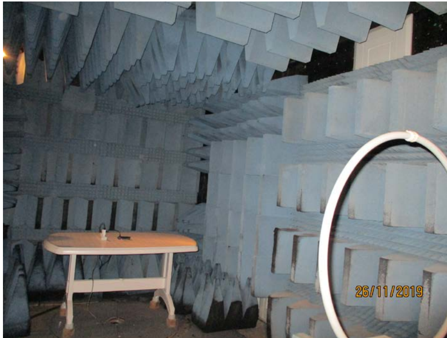
Figure 6. Radiated Emission Test, 0.009-30MHz
