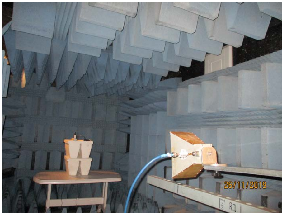
Figure 9. Radiated Emission Test, 1-18GHz
