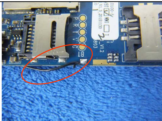
BT - Antenna View
