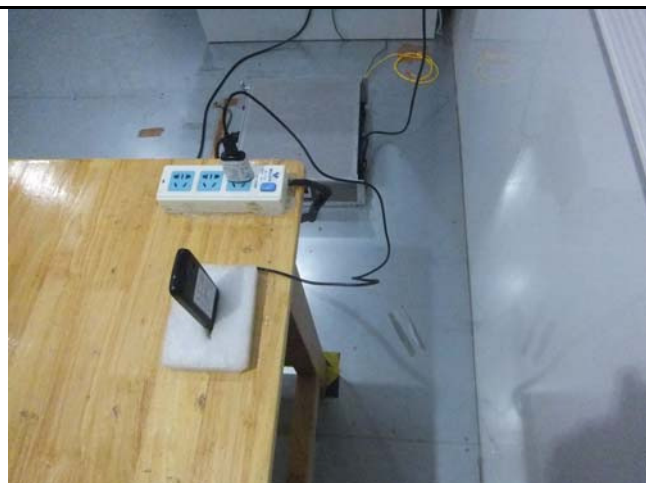
Conducted Emissions Test Setup Side View
