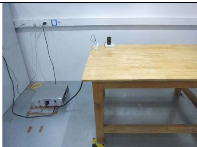
Conducted Emissions Test Setup Front View
