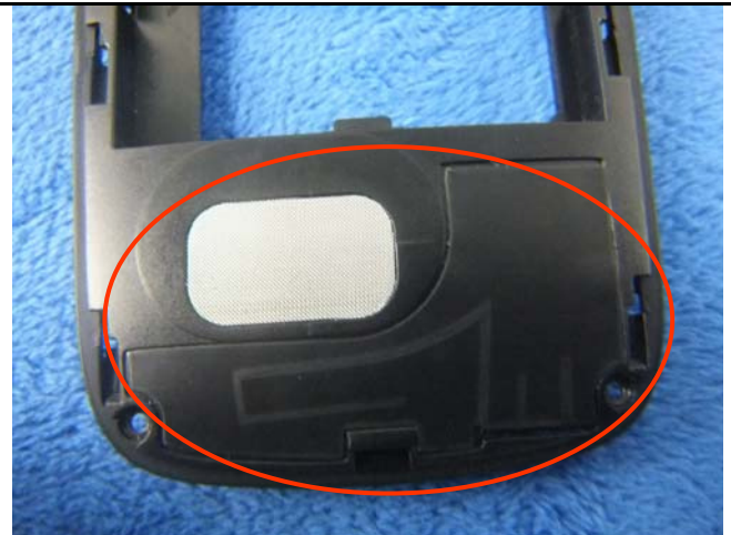
GSM/PCS Antenna View
