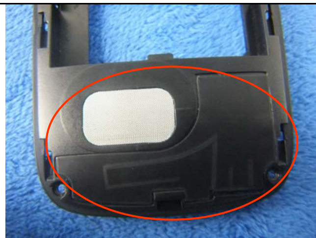
GSM/PCS Antenna View
