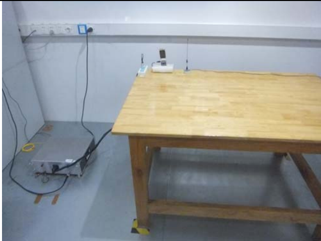
Conducted Emissions Test Setup Front View
