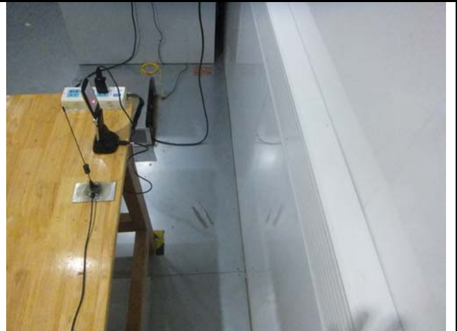
Conducted Emissions Test Setup Side View
