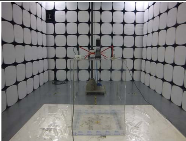
Radiated Spurious Emissions Test Setup Below 1GHz
