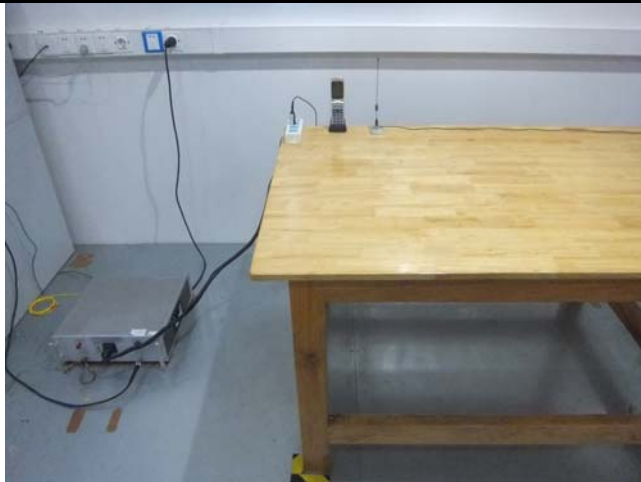
Conducted Emissions Test Setup Front View
