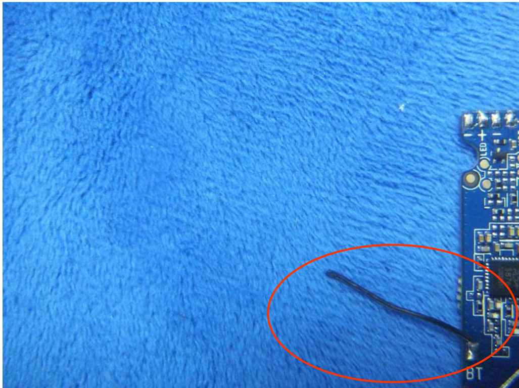
BT-FDD Antenna View
