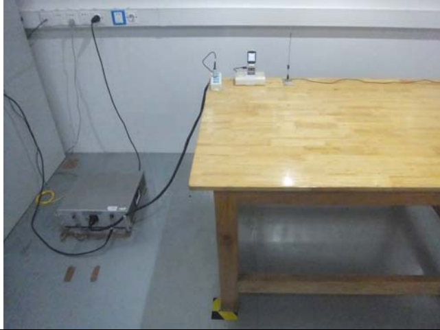
Conducted Emissions Test Setup Front View
