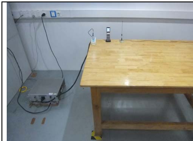
Conducted Emissions Test Setup Front View
