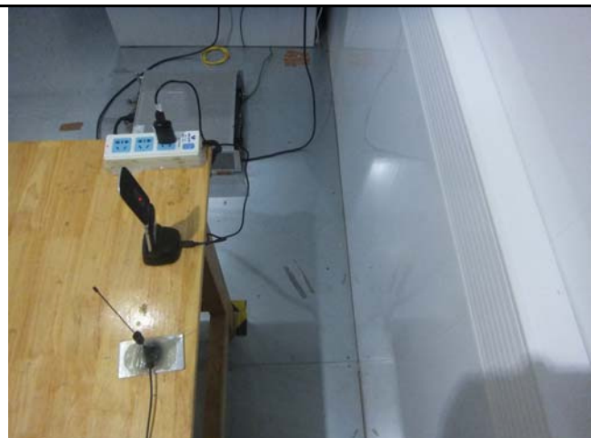
Conducted Emissions Test Setup Side View
