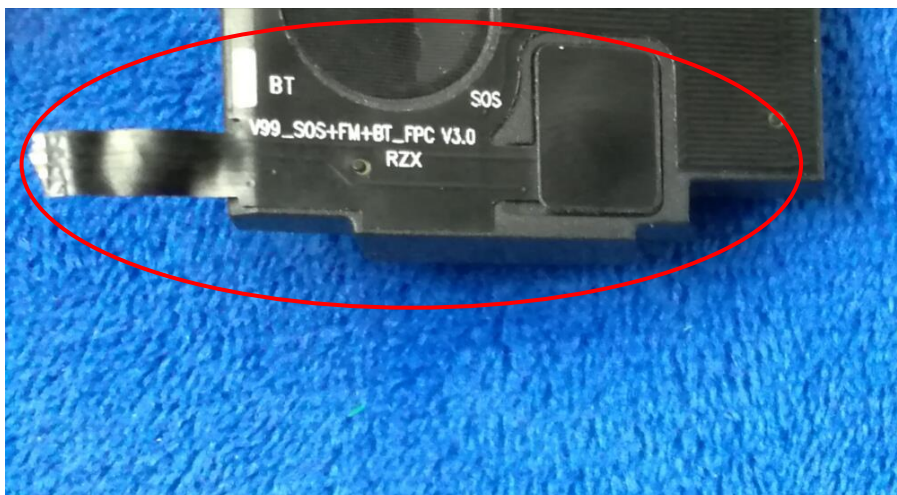
BT - Antenna View
