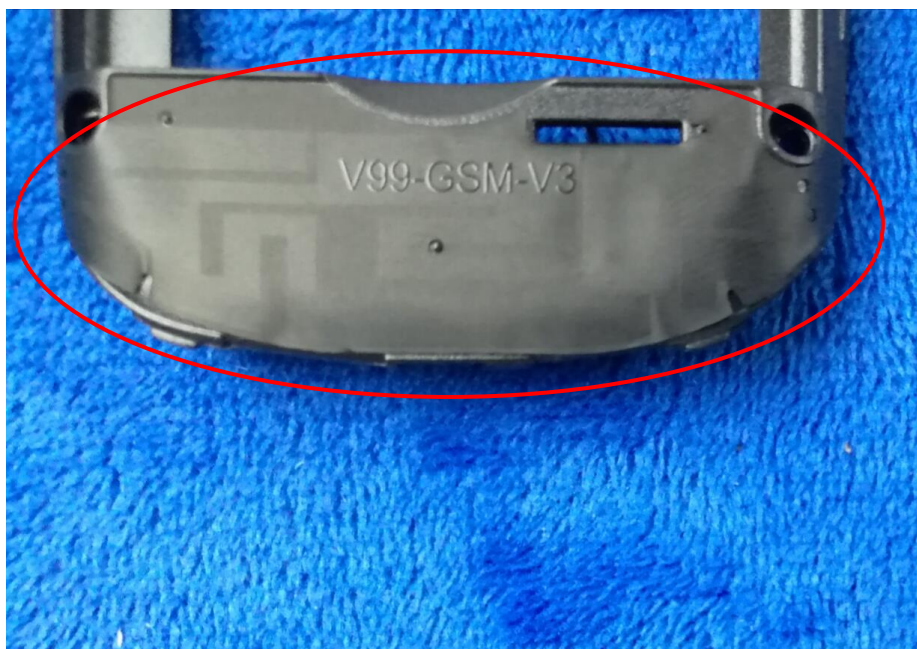
GSM/PCS/UMTS-FDD - Antenna View
