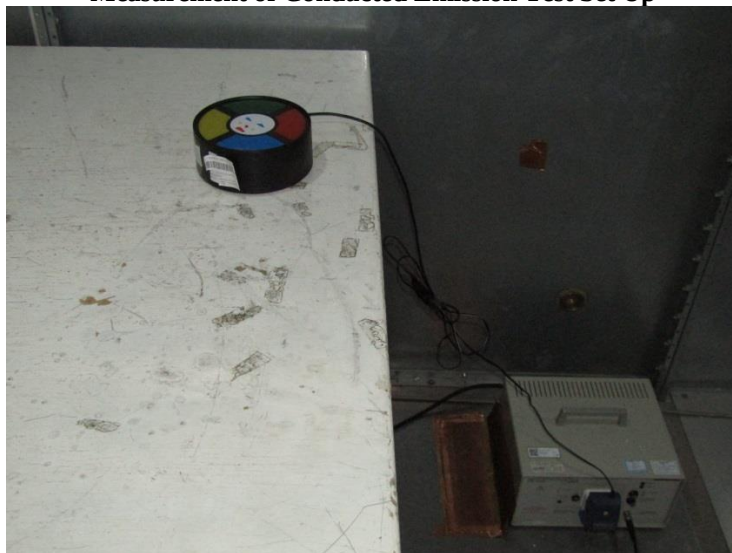
Measurement of Conducted Emission Test Set Up
