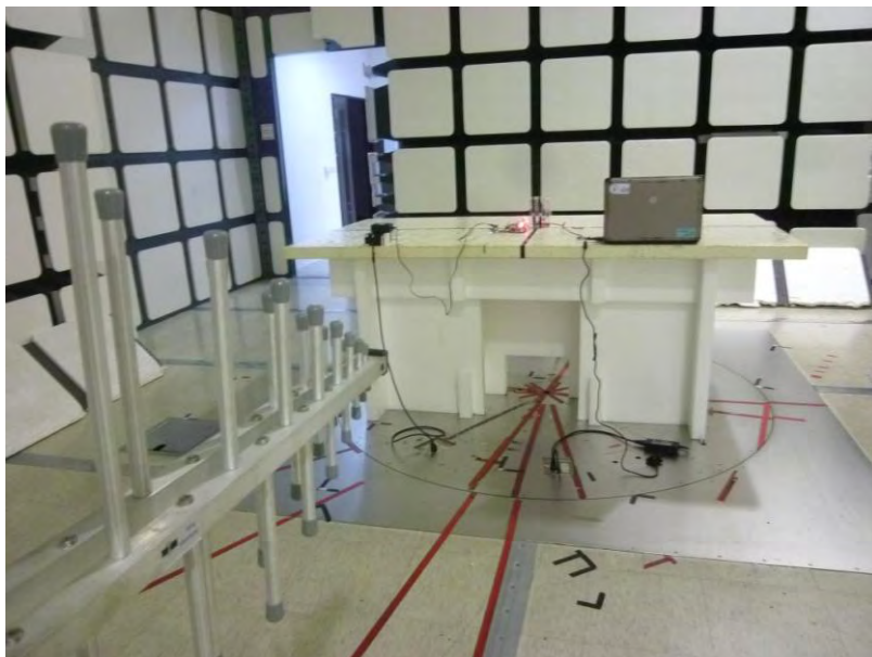
Below 1GHz _ Rear View _ Antenna Model : EDA-1713-25GC1-A14
