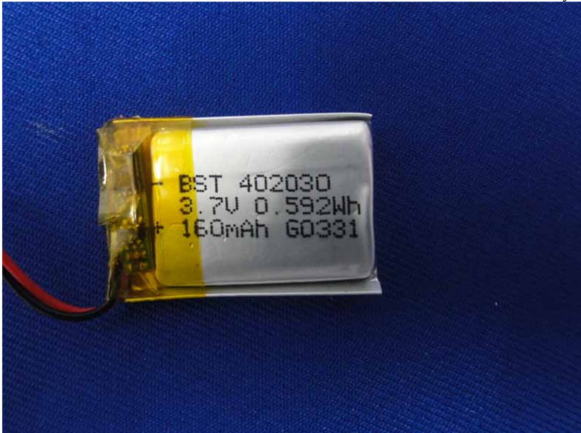
Figure 4 Battery of the EUT
