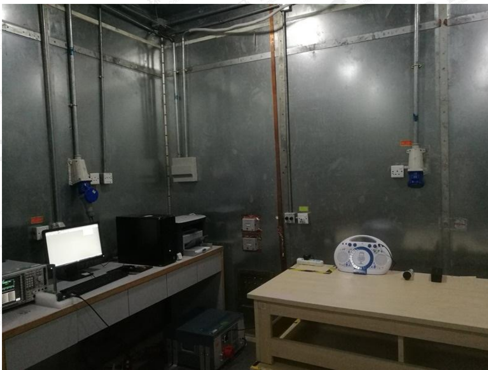
FCC RADIATED EMISSION TEST SETUP
