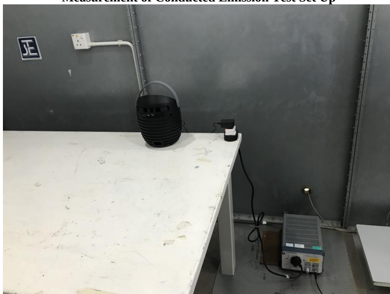
Measurement of Conducted Emission Test Set Up
