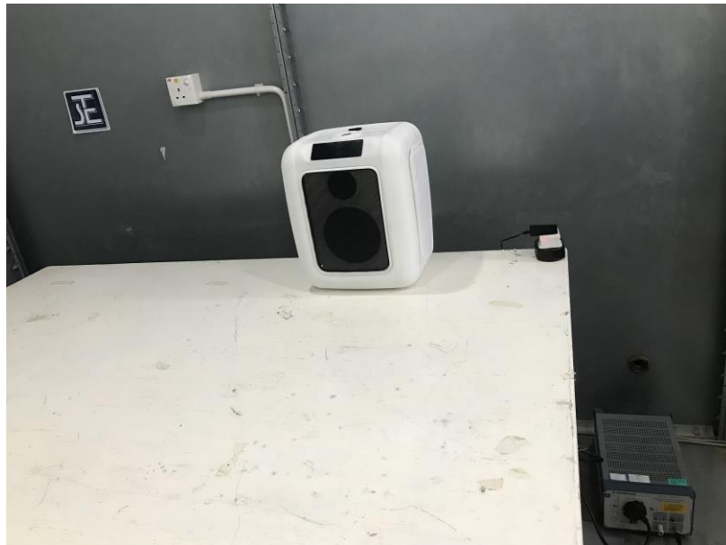
Measurement of Conducted Emission Test Set Up
