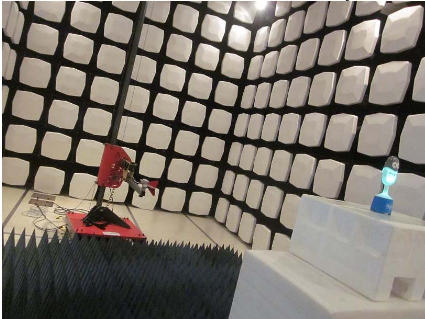
Measurement of Radiated Emission Test Set Up
