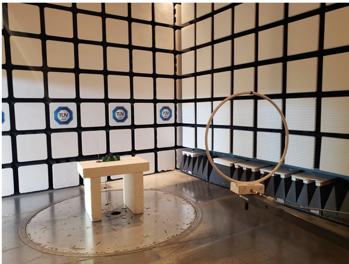
Figure 2 – Radiated Emissions Setup 9kHz – 30MHz
