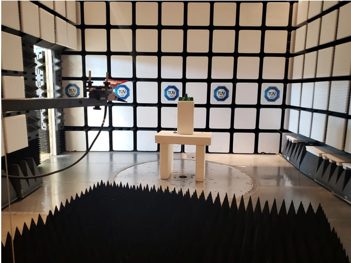
Figure 4 – Radiated Emissions Setup 1GHz – 6GHz
