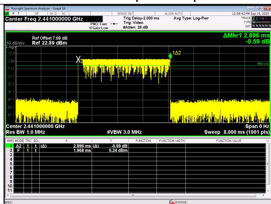
Pulse Width 8DPSK_3-DH5
