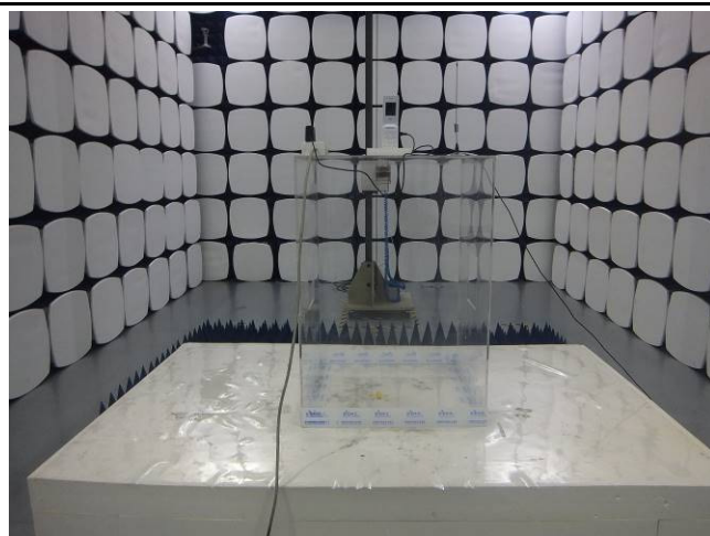
Radiated Spurious Emissions Test Setup Above 1GHz
