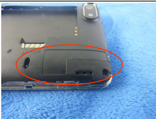
WIFI/BT/BLE/GPS - Antenna View
