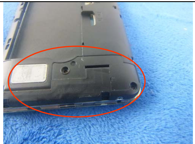
GSM/PCS/UMTS-FDD Antenna View
