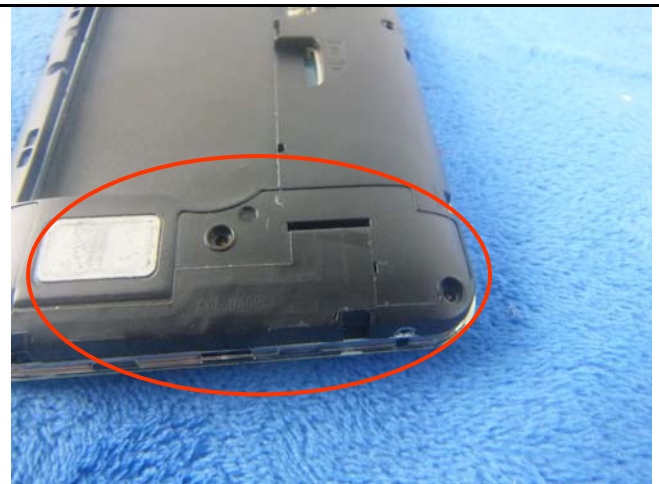
GSM/PCS/UMTS-FDD Antenna View
