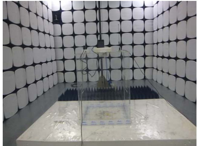
Radiated Spurious Emissions Test Setup Above 1GHz
