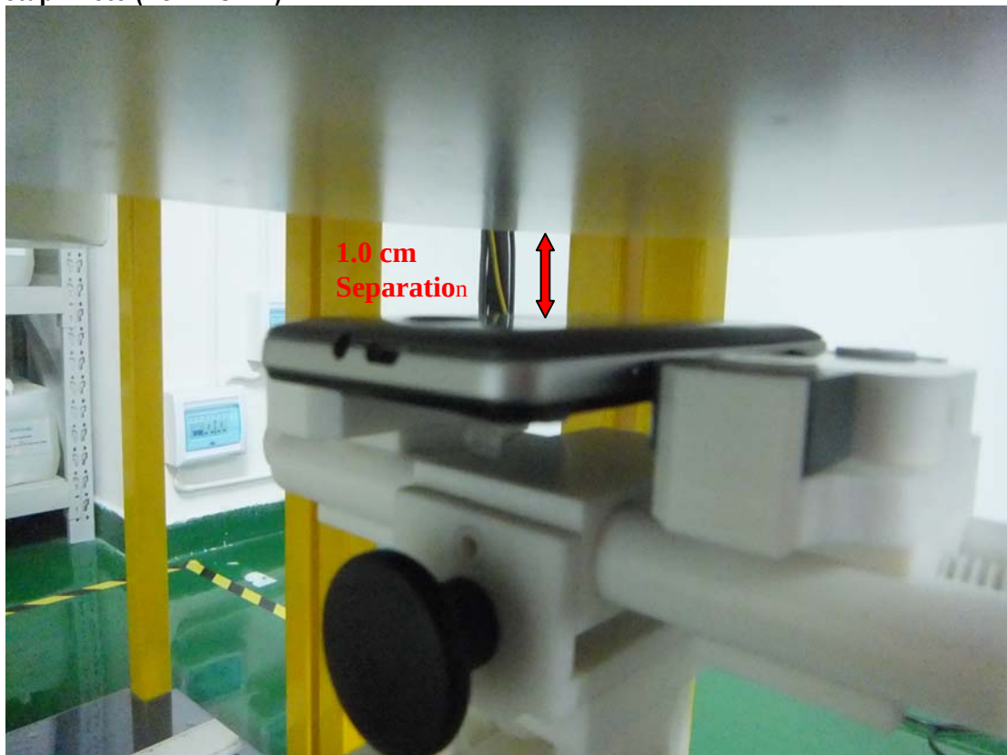
Body Setup Photo (LCD DOWN)
