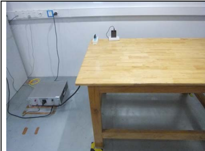
Conducted Emissions Test Setup Front View
