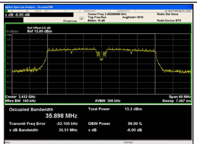
802.11n40 6dB Bandwidth - High CH 2452
