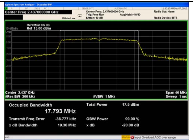
802.11n20 20dB Bandwidth - Mid CH 2437
