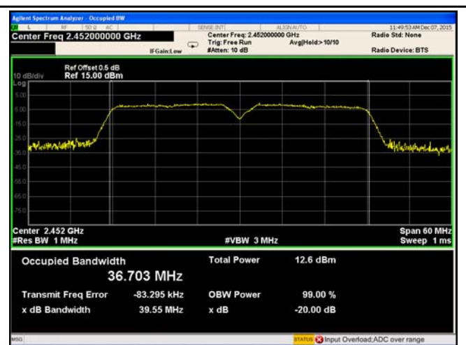
802.11n40 20dB Bandwidth - High CH 2452
