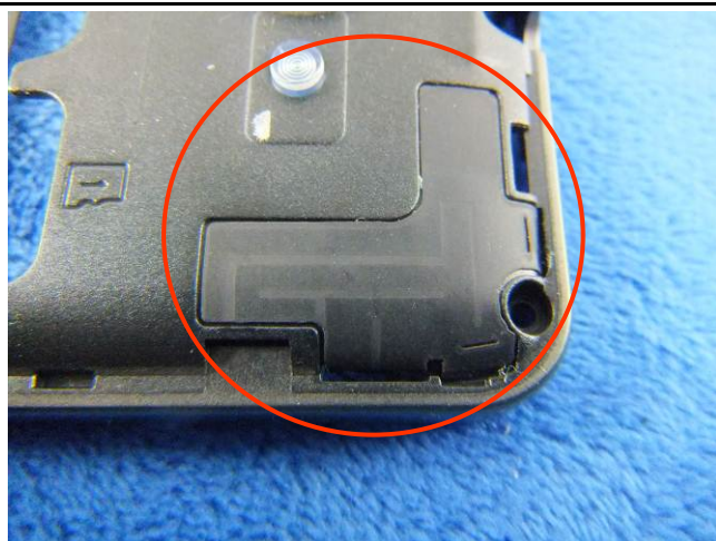
WIFI/BT/BLE/GPS - Antenna View
