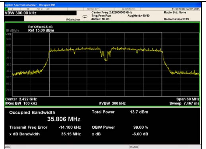
802.11n40 6dB Bandwidth - Low CH 2422
