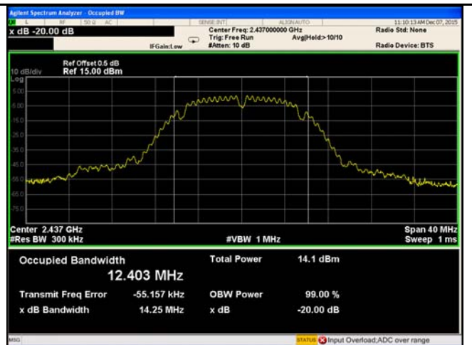
802.11b 20dB Bandwidth - Mid CH 2437
