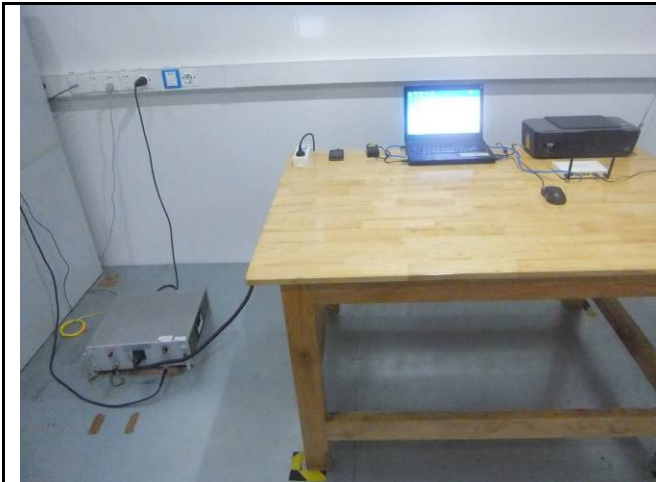
Conducted Emissions Test Setup – Front View
