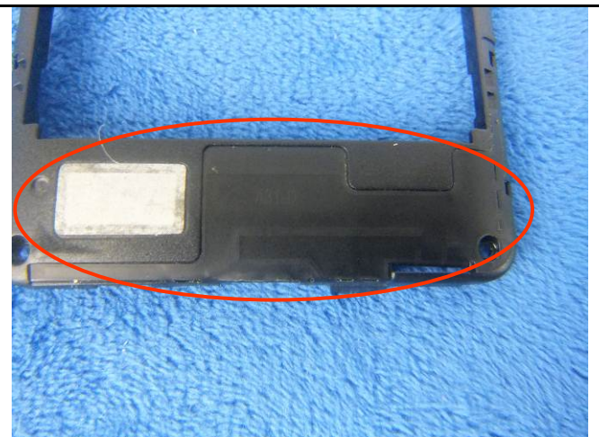
GSM/PCS/UMTS-FDD Antenna View
