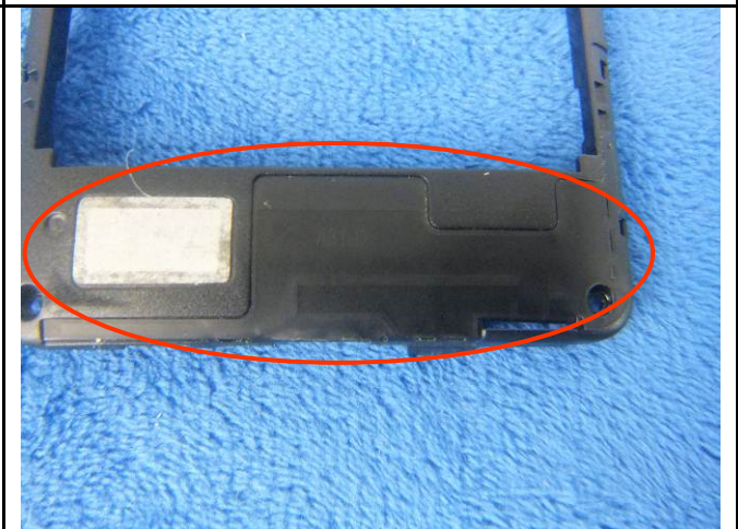
GSM/PCS/UMTS-FDD Antenna View
