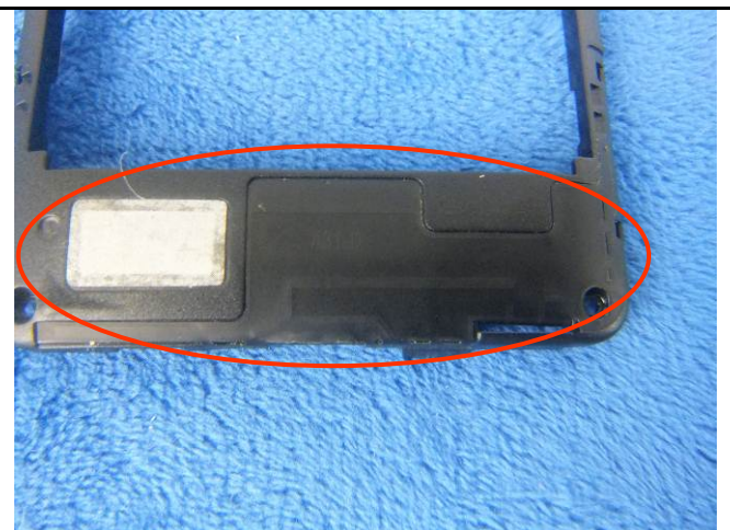
GSM/PCS/UMTS-FDD Antenna View
