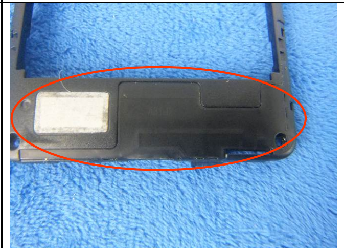
GSM/PCS/UMTS-FDD Antenna View
