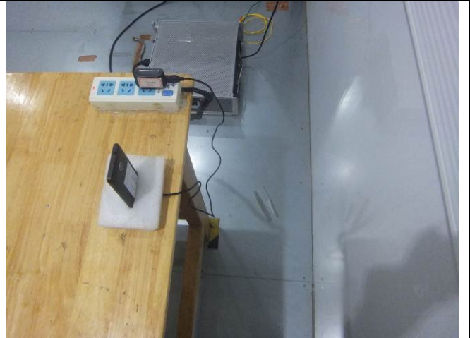
Conducted Emissions Test Setup Side View
