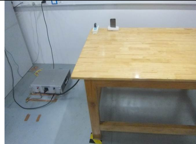
Conducted Emissions Test Setup Front View
