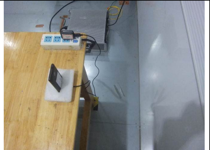
Conducted Emissions Test Setup Side View
