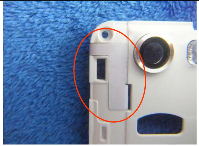
LTE Antenna View
