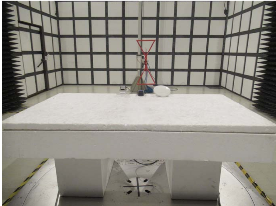
Radiated Disturbances Rear Side (Below 1GHz)
