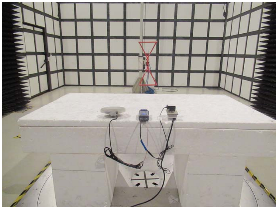
Radiated Disturbances Rear Side (Below 1GHz)
