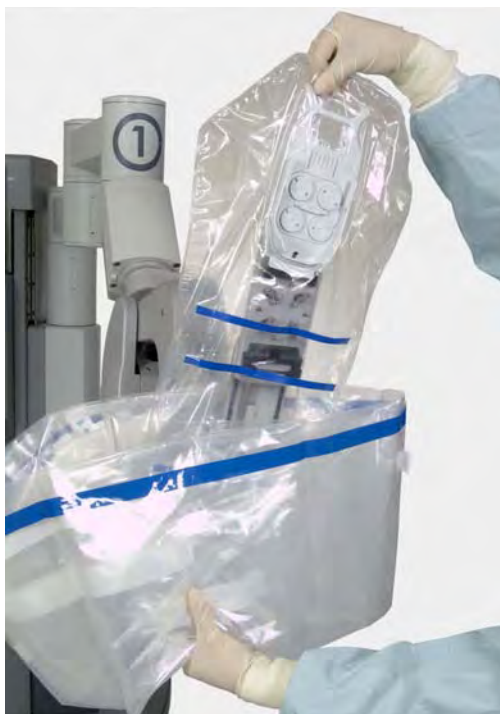
Figure 6.9 Lowering the drape over the insertion axis
