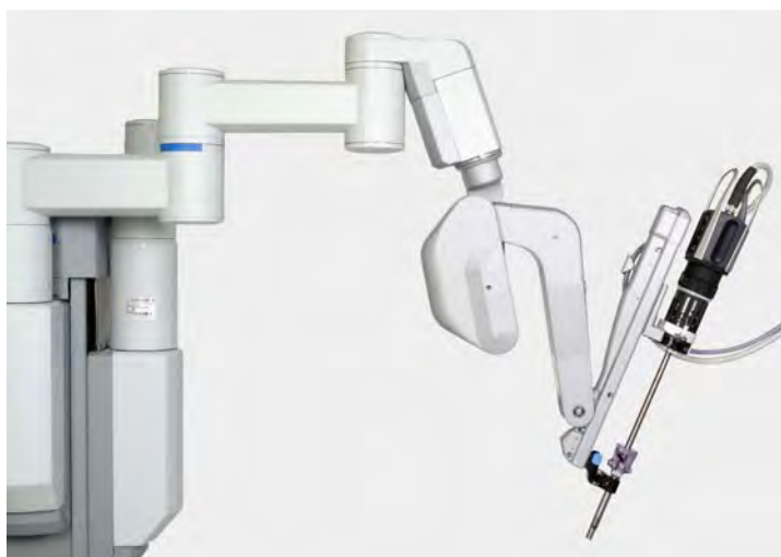
Figure 2.14 Camera arm with attached endoscope
