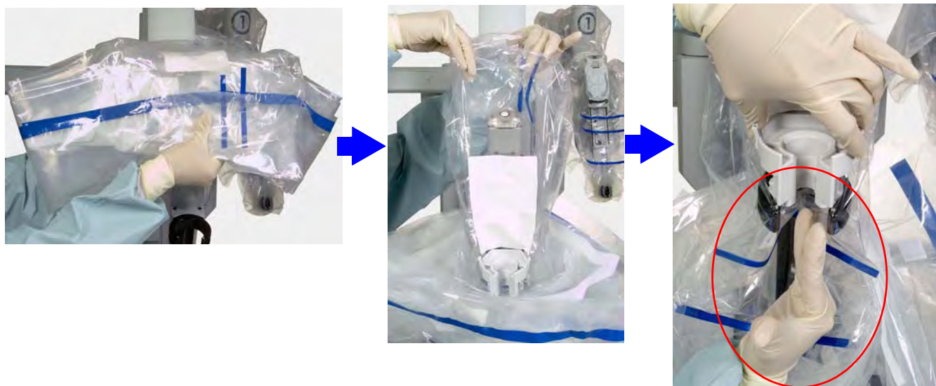
Figure 6.16 Lower over insertion axis, install sterile adapter
