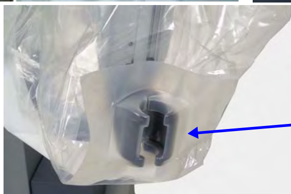
Figure 6.12 Seat the cannula mount molding
