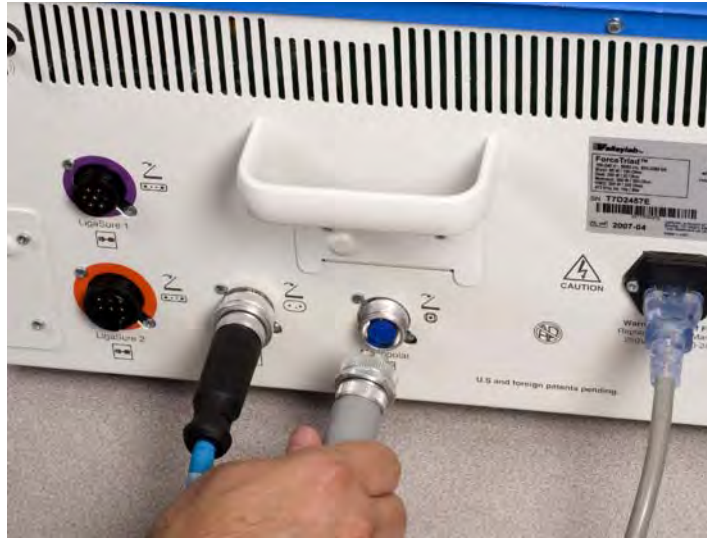
Figure 4.13 Auxiliary device connection (back of ESU)
