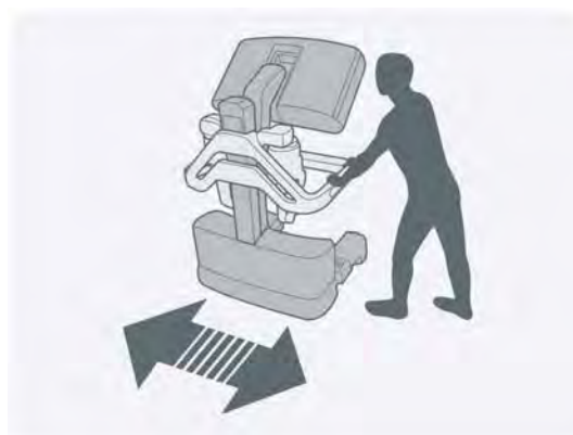
Move Surgeon Console using handles on side
