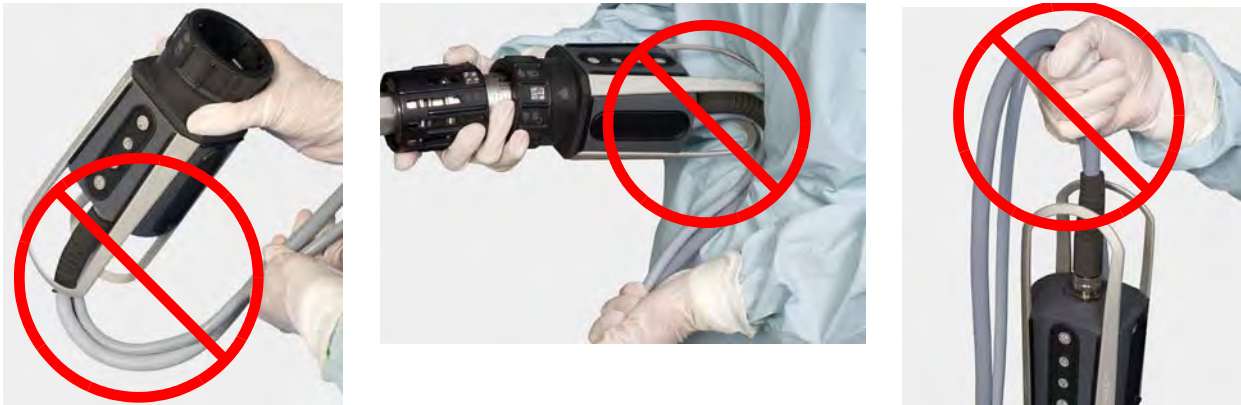
Figure 7.4 Examples of mishandling camera head cables
