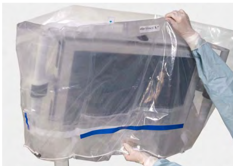
Figure 6.24 Lower the drape over the monitor
