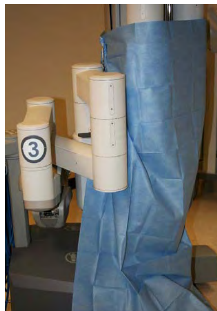
Figure 6.6 Secure with towel clamp | Clamp opposite of instrument arm 3
