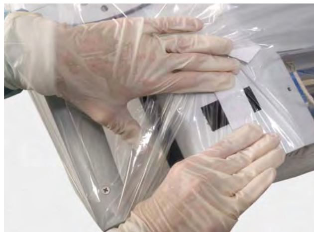
Figure 6.28 Secure Velcro straps on sides and rear
