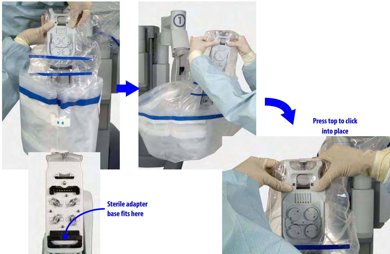
Figure 6.10 Insert base, press top to install sterile adapter
