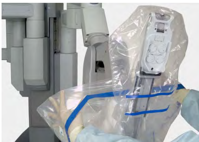
Figure 6.11 Stretching the drape along the arm
