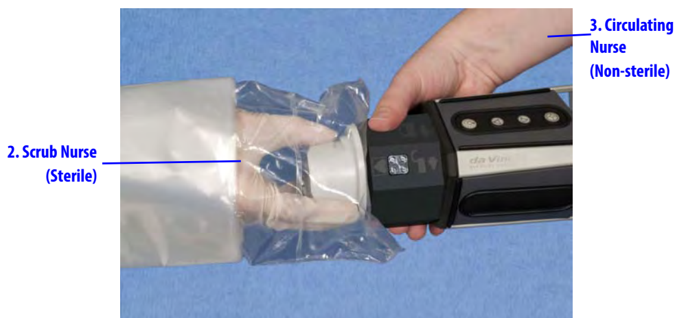
Figure 6.21 Attaching camera head to sterile adapter
