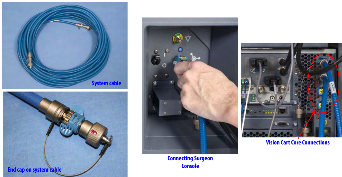
Figure 4.1 Sample system cable and connections
