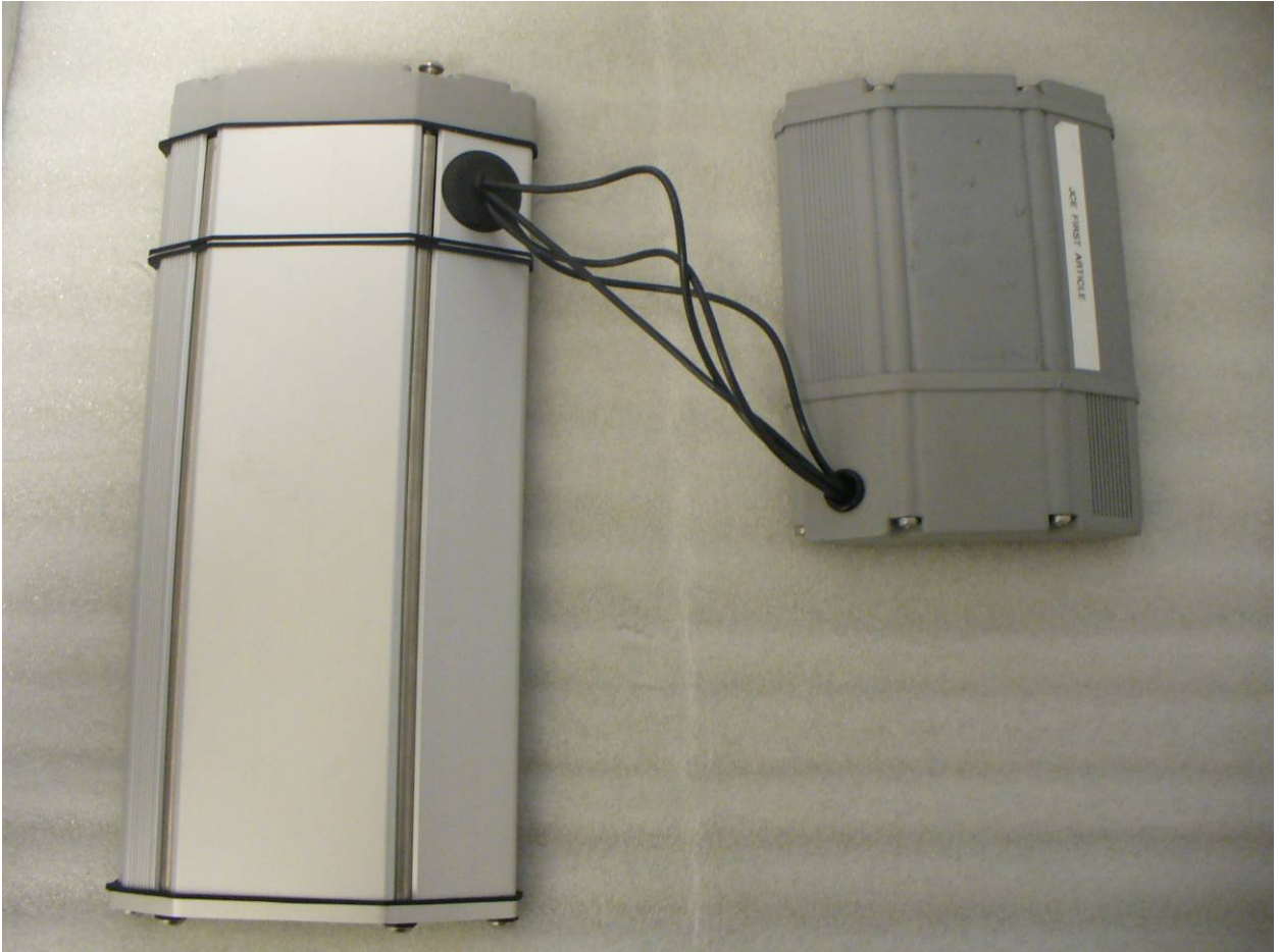
Figure 1: GTCU: Globe Tracker Communication Module (GTCM) and Globe Tracker Antenna Module
