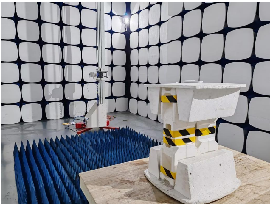
Radiated Emission (Above 1GHz)
