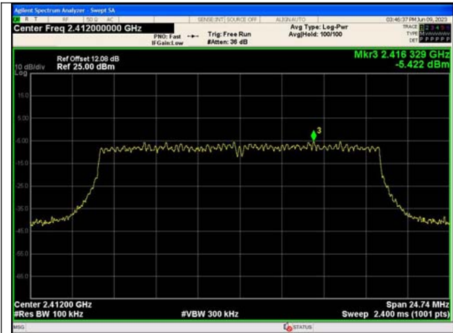
In-Band Reference Level IEEE 802.11g_Channel 1_20MHz_Antenna 0
