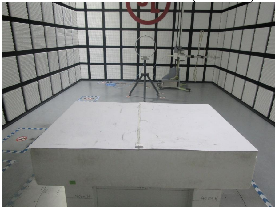
RADIATED RF MEASUREMENT SETUP (Below 30MHz)
